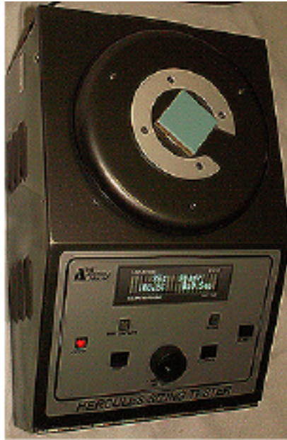
Figure 3-1A: This figure demonstrates the white side of the tile facedown on the specimen opening prior to performing the standardization procedure.
