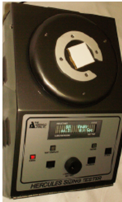
Figure 3-1: This figure demonstrates the green side of the tile facedown on the specimen opening prior to performing the standardization procedure.
