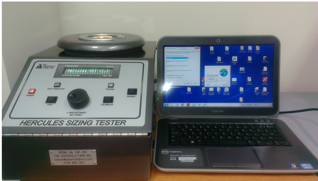
Figure 1-1: This photo of the new Hercules Sizing Tester shows the end of a test. The right side illustrates one of the features -- an RS-232 port for transmitting data to a computer.
