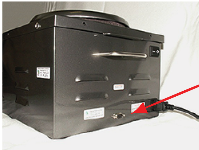
Figure 9-9C: The RS-232 Data Port is a 9-pin port located on the rear side of the HST. Use only with RS-232 cables or adapters.
