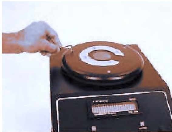
Figure 5-1: Access to the air filter is obtained by removal of three screws around the outside of the optical cover plate.
