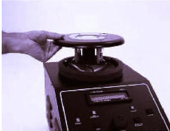
Figure 5-3: When replacing the optical assembly, be certain to position the unit in its original location. To obtain the proper position align the lamp bulbs in the 4 o'clock and 10 o'clock positions.
