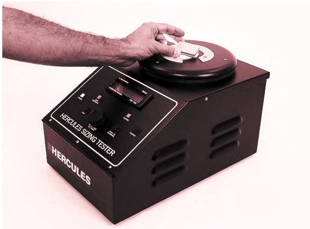
Figure 3-1: This figure shows the operator placing the white tile face onto the specimen opening prior to performing the Standardization procedure.
