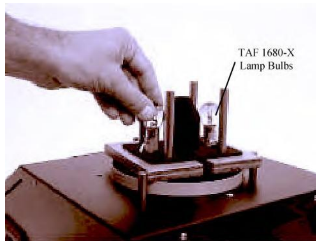
Figure 5-6: Bulb Removal -The operator is pressing down and twisting the bulb to remove it from its socket.
