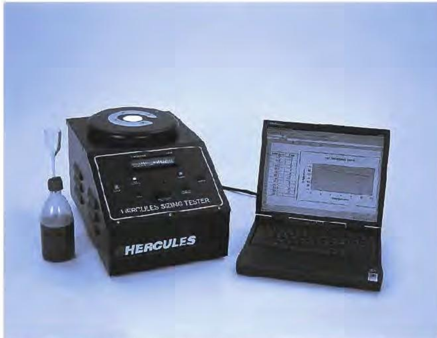
Figure 1-1: This photo of the new Hercules Sizing Tester shows the end of a test. Next to the unit is a bottle for dispensing the 10-m l ink sample. The right side illustrates one of the new features -- an RS-232 port for transmitting data to a computer.
